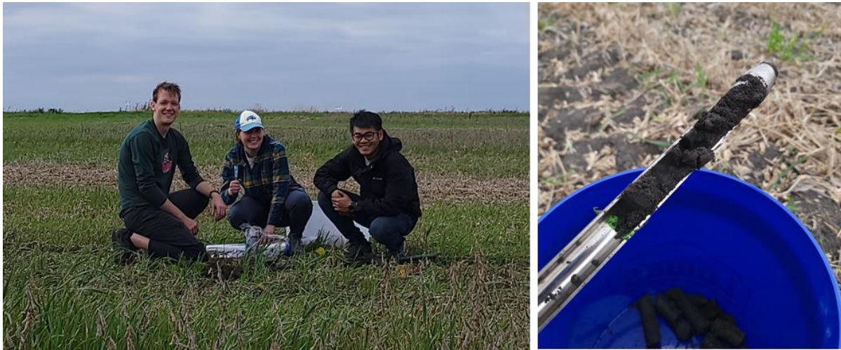
Figure 3. The WQRL research team collected Uhland cores and topsoil samples in the fall of 2021 for plot level nutrient and soil health analysis. Three Uhland core samples were collected per plot, then processed and composited in the lab for analysis. The topsoil samples were divided into 0-6" and 6-12" increments in the field, with 4-6 samples collected at each plot depending of the diameter of the probe used for collection to ensure an adequate volume of sample for analysis.
