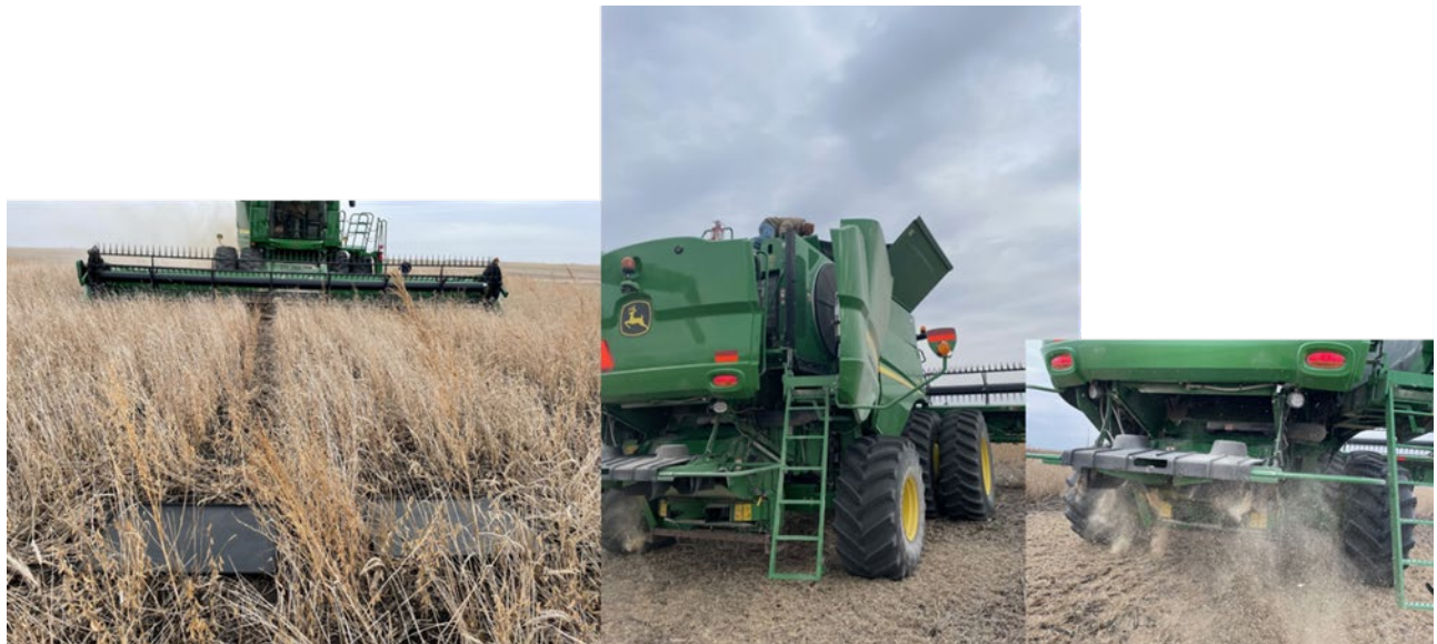
Figure 2. Measuring header, grain tank, and thresher losses of waterhemp seeds at harvest in a soybean field in Iowa, 2022.
