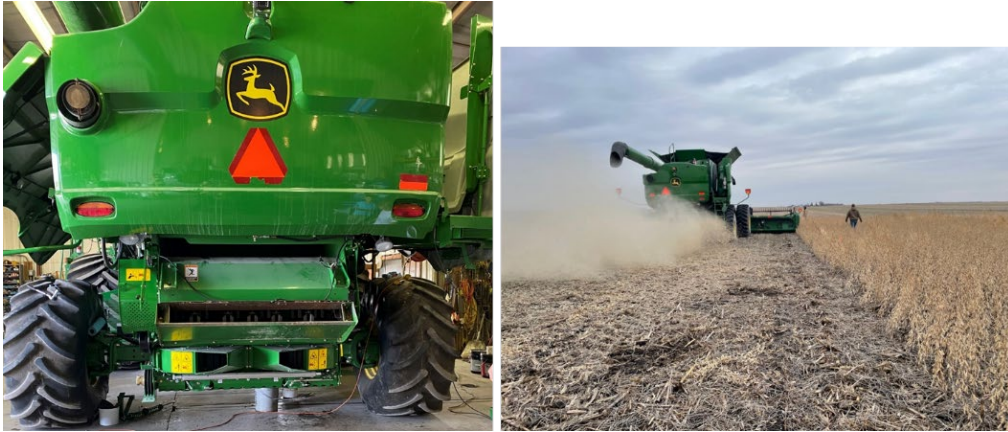
Figure 1. Redekop seed destructor (high-impact mill) attached to a John Deere S680 combine in a soybean field at harvest in Dayton, Iowa, 2022.
