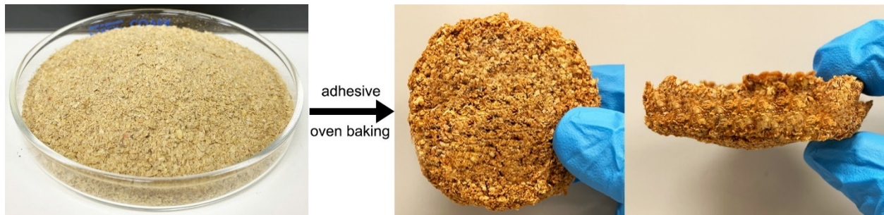
Figure 2. Photographs showing soy hull particles being processed into a cylindrical solid product after mixing with the adhesive and oven baking.
