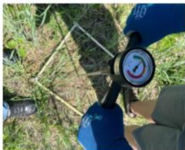
Testing soil strength with cone penetrometer
