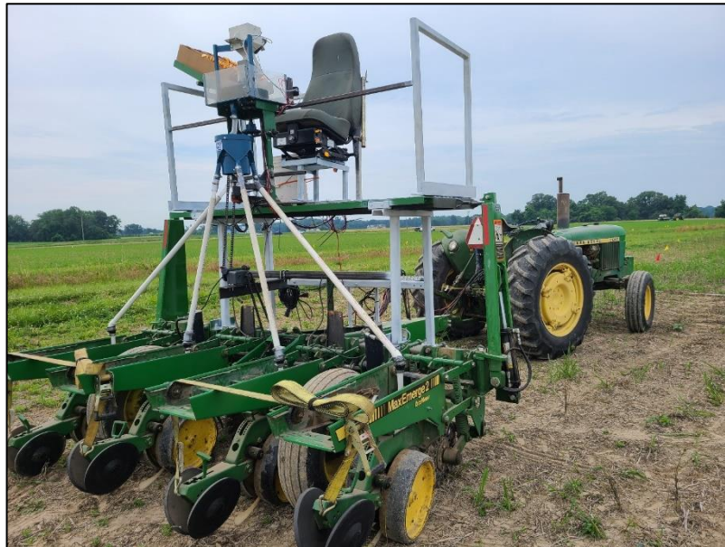
Figure 1. Modified no-till planter fabricated in 2021 for no-till planting of all plots in the soybean variety trials.
