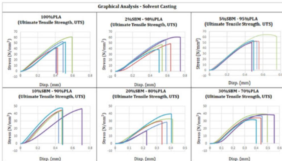
Figure 10: Summary of tensile stress versus displacement behavior of composites
