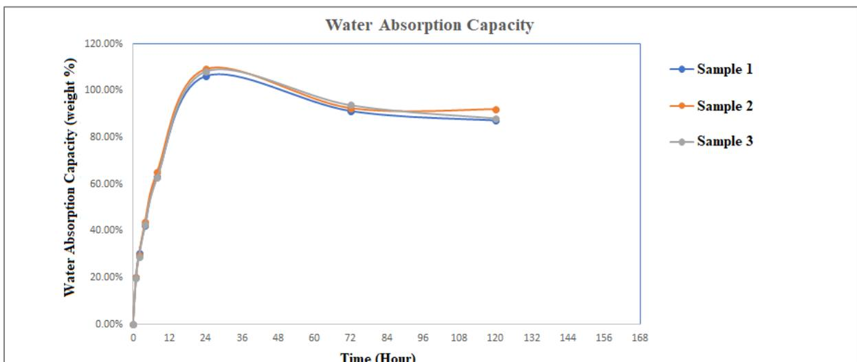
Figure 8: Water absorption results of different samples
