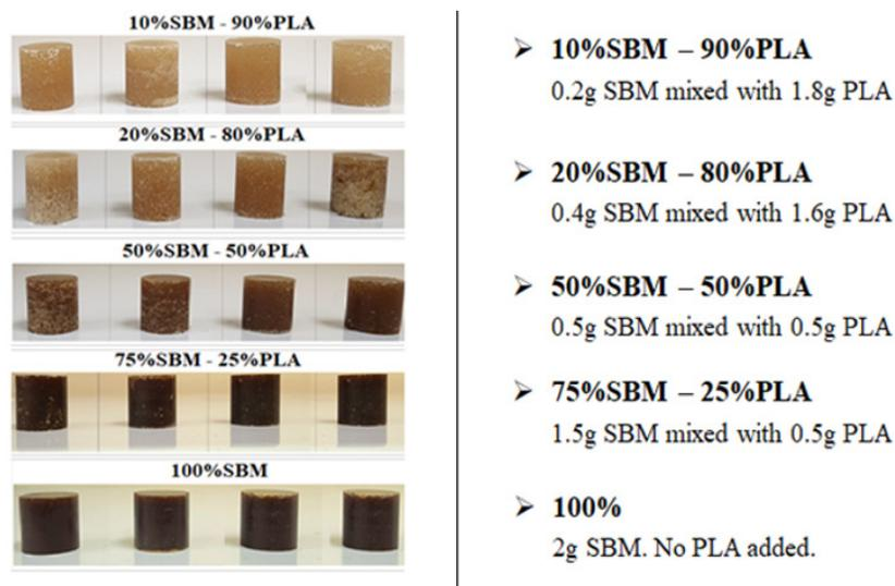
Figure 4: Different samples synthesized during this study
