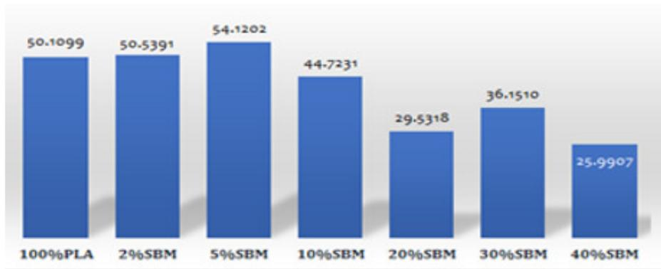
Figure 11: Summary of tensile strength behavior of composites (all values are in MPa).
