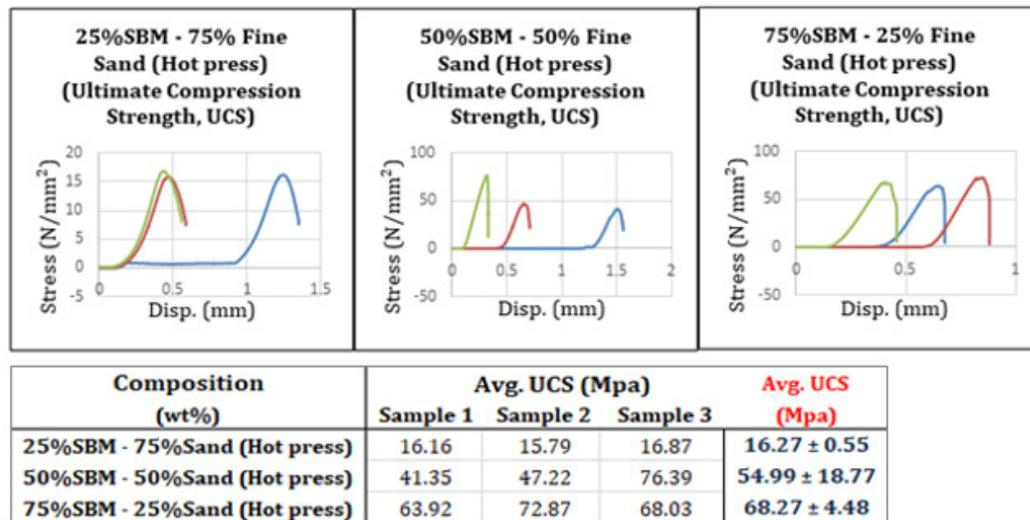
Figure 12: Summary of mechanical performance of SM-based composites with sand
