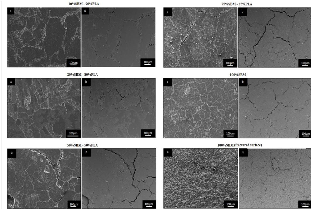
Figure 7: SEM micrographs of PLA-SBM composites.
