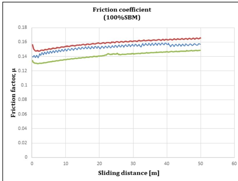
Figure 9: Friction coefficient versus sliding distance of hot pressed Soybean Meal.
