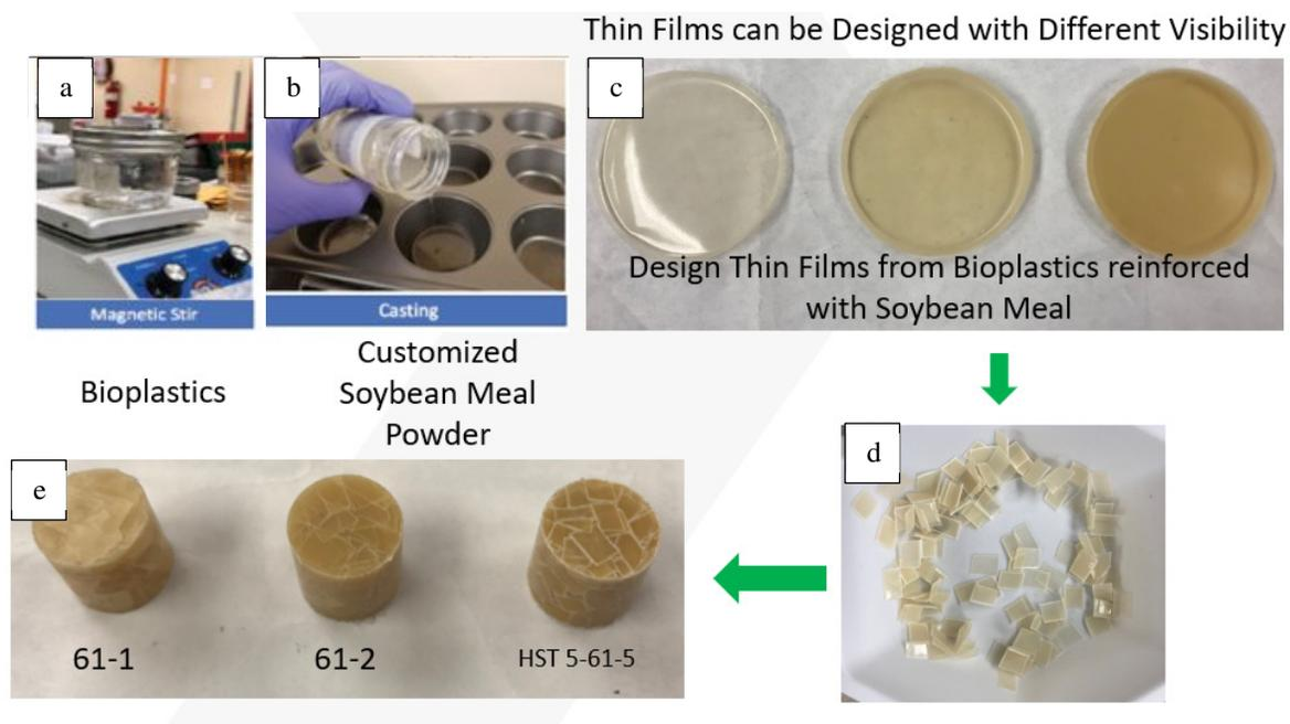
Figure 2: Digital pictures of, (a) stirring process), (b) liquid ink (images courtesy: Saud et al. JMPEP), and (c) solvent-cast films, (d) machined coupons, and (e) hot-pressed samples (pictures courtesy: Dr. Zhang).
