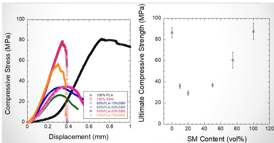
Figure 5: Plot of, (a) compressive stress versus displacement, and (b) ultimate compressive strength versus Soybean Meal Content.
