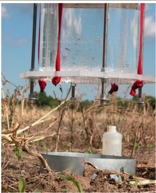
Figure 1 A Cornell Sprinkler Infiltrometer being lowered down to begin simulated rain inside a 24.1 mm I.D. metal ring installed 7.5 cm into the soil.
