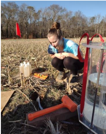
Figure 2 Collecting the first 5 liters of runoff from a simulated rain event using distilled water and the Cornell sprinkler infiltrometer.
