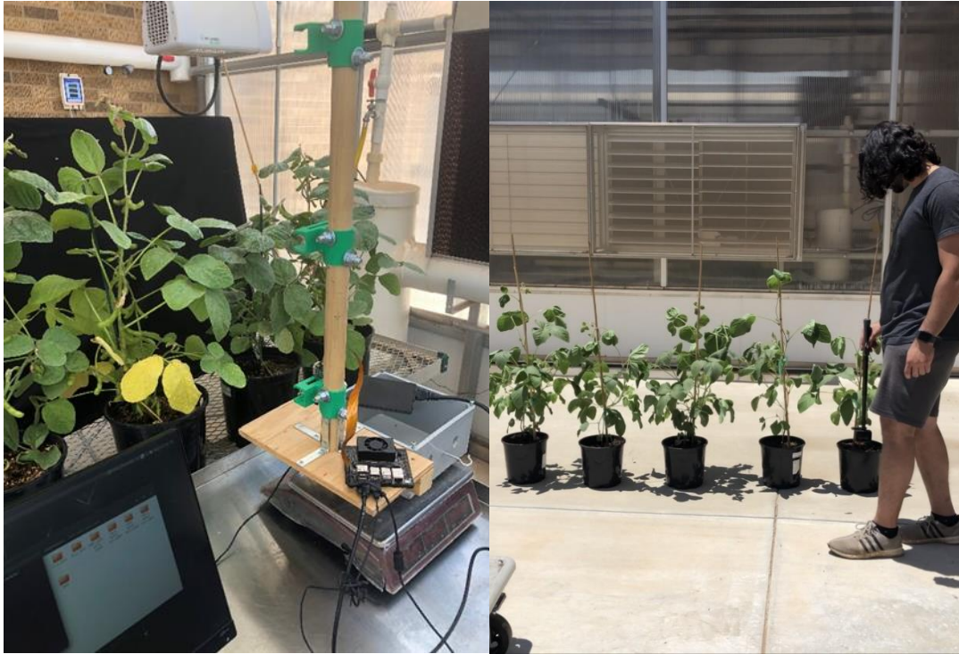
Figure 7. Imaging system test in a greenhouse to set camera parameters and check the ability to capture and record high-quality images at 60 frames per second.
