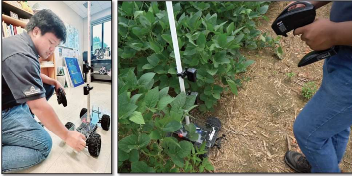
Figure 3. GoPro Hero11 cameras mounted on a Traxxas Hoss ® 4x4 VXL conveyor (left) the imaging technique for soybean flowers in between rows using our conveyor (right) (at WTREC)
