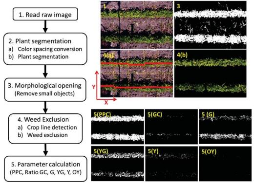
Figure 2. Summary of the new image processing algorithm developed for soybean plot images.
