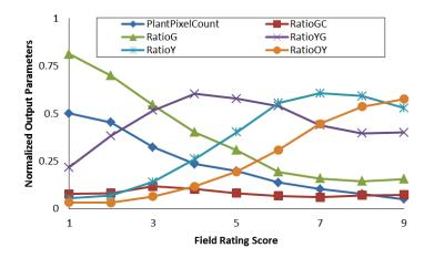
Figure 3. The relationship between the six color parameters extracted from the soybean plot images and their IDC visual rating in the field.
