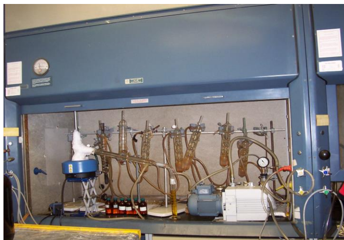
Figure 5: Vacuum Distillation setup used for determining boiling ranges of soybean oil and high oleic soybean oil esters.
