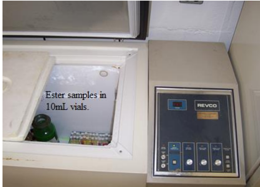
Figure 4: Photograph freezer with ester samples in 10mL vials used for pour point and cloud point determinations.
