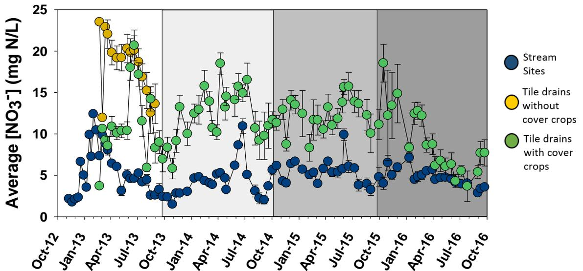
**Figure 3.** SDW tile drain NO<sub>3</sub><sup>-</sup> concentrations have been lower since saturating the watershed with cover crops in October 2013 and in spring/summer 2016 the tile drain NO<sub>3</sub><sup>-</sup> concentrations were almost as low as the stream NO<sub>3</sub><sup>-</sup> concentrations.
