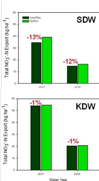
Figure 7. Comparison of total nitrate export calculated from SUNA data vs. export modeled using grab samples.
