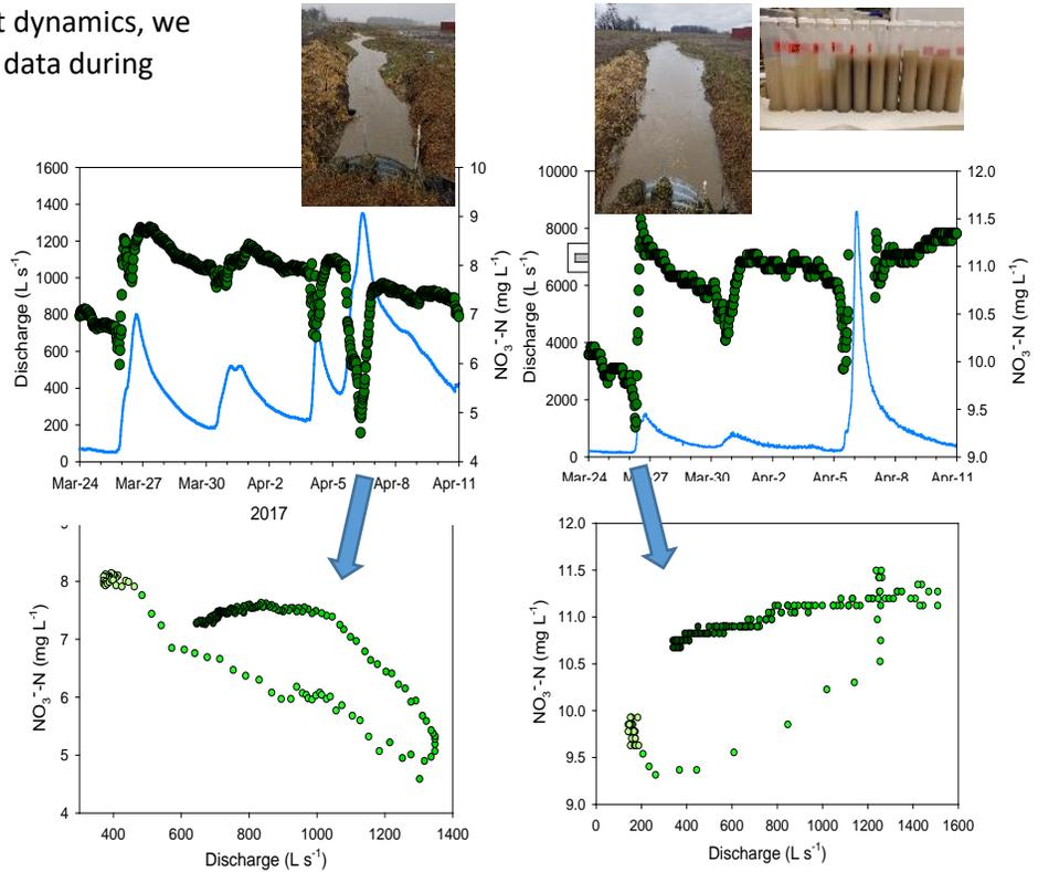
Figure 8. Trends in mean daily nitrate concentration (green dots) and discharge (blue line) show that concentrations can either increase with or be diluted by discharge during a storm and that hysteresis may occur, whereby patterns on the ascending and descending limbs of a storm may differ.
