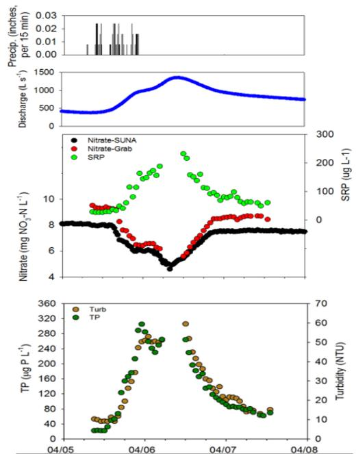
Figure 10. Precipitation, hydrograph, nutrient, and turbidity values for a storm at the outlet of SDW on April 5, 2017
