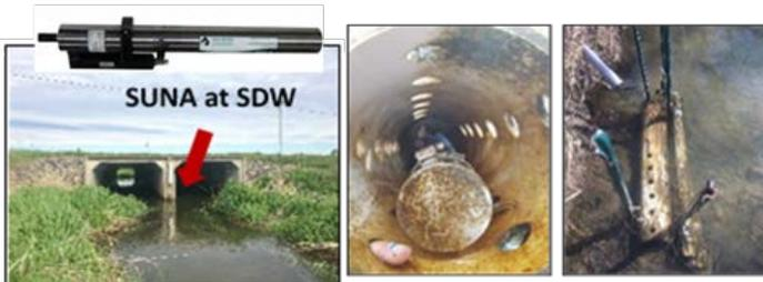
Figure 9. Images of SUNA nitrate sensor deployment.
