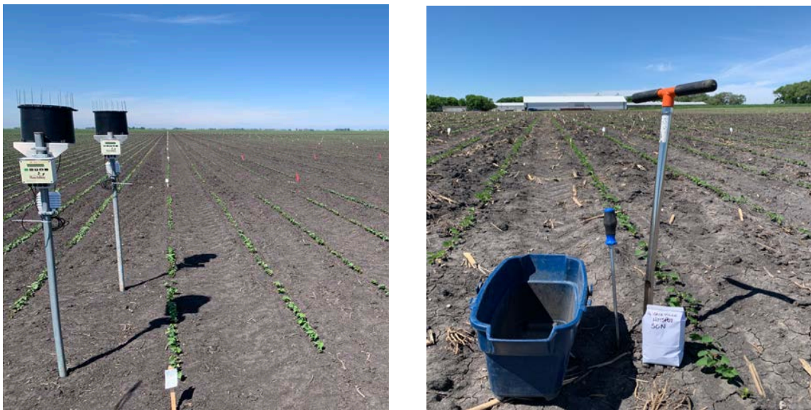
Figure 6. Weather stations were installed at each field site and soil cores were collected for soil characterization.
