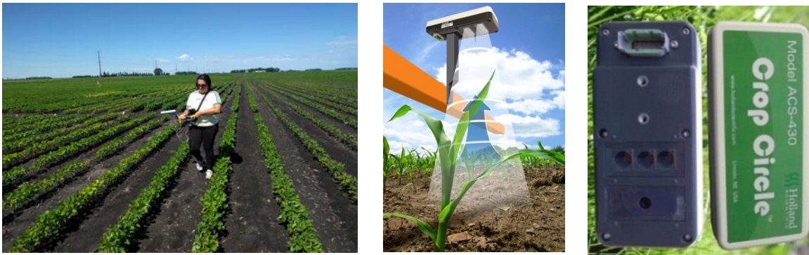
Figure 8. Ground-based crop reflectance data being collected with an active crop canopy sensor.
