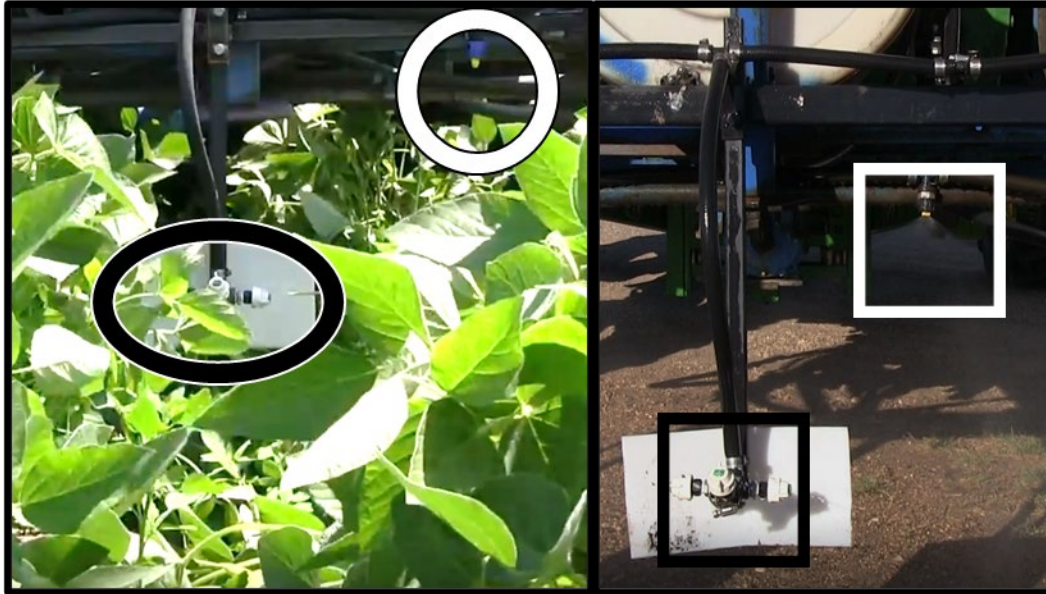
Figure 1. Configuration of the tractor-mounted hydraulic-powered plot sprayer used to apply fungicides in this experiment. Note that two different within-the-canopy booms were built to allow application down the center of both 22 (Crookston study site) and 30 inch (Staples study site)-spaced soybean rows. The within-the-canopy nozzle body (black circle/square) rode approximately 12 inches from the soil surface and the over-the-top nozzles (white circle/square) rode approximately 8 inches above the soybean canopy.
