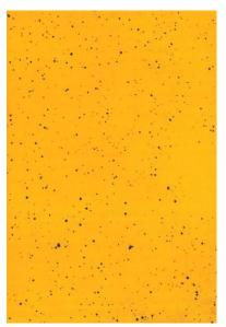
Coverage: 2.84% Droplet density: 21.8 droplets/cm<sup>2</sup> VMD: 269  $\mu m$
