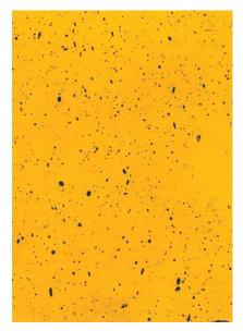
Coverage: 4.22% Droplet density: 43.0 droplets/cm<sup>2</sup> VMD: 308  $\mu m$
