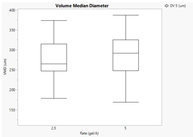
*Figure 3.* Box plot showing distribution and volume median diameter (VMD) for spray droplets applied at volumes of 2.5 and 5.0 gallons per acre.
