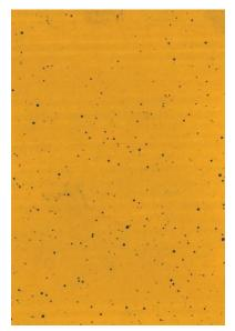
Coverage: 1.35% Droplet density: 10.9 droplets/cm<sup>2</sup> VMD: 283  $\mu m$
