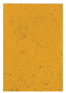
Coverage: 3.51% Droplet density: 37 droplets/cm<sup>2</sup> VMD: 260 µm
