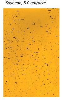
Coverage: 3.49% Droplet density: 36 droplets/cm<sup>2</sup> VMD: 292 µm
