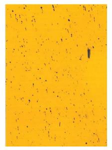
Coverage: 2.99% Droplet density: 21.9 droplets/cm<sup>2</sup> VMD: 292  $\mu m$
