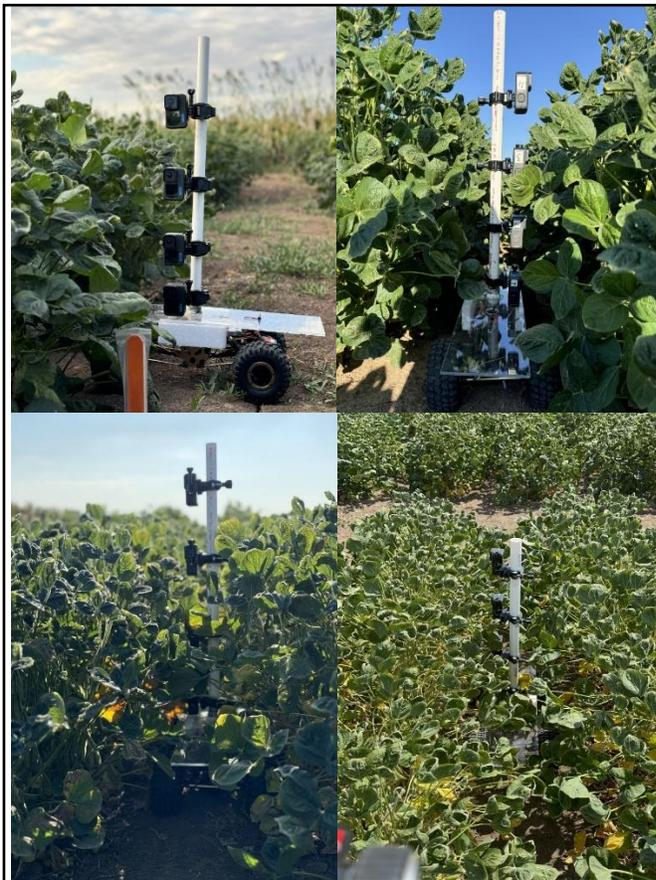
**Figure 12.** RC car crawler mounted with GoPro Cameras. Texas Tech University
