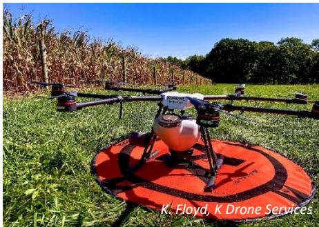
Figure 1. DJI drone equipped with hopper and spin spreader.
