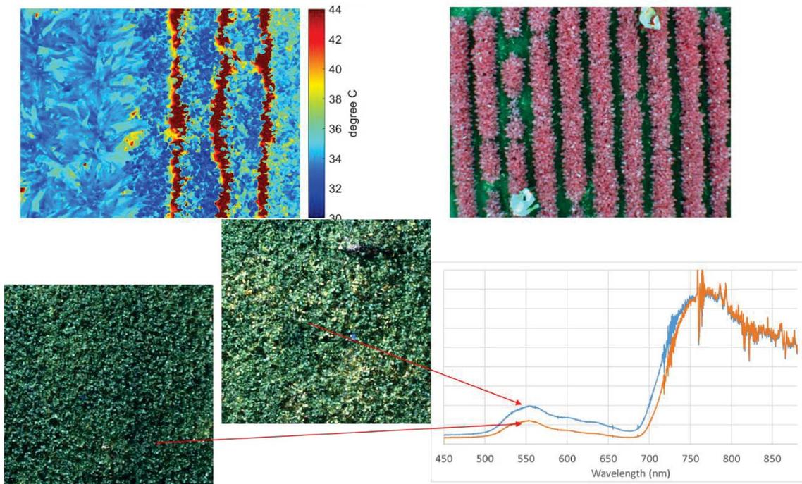
Figure 6. Picture showing the team working in the Spidercam field (soybean part) for data collection; and example soybean canopy images (thermal infrared and color-infrared) and spectral reflectance from the Spidercam instruments.
