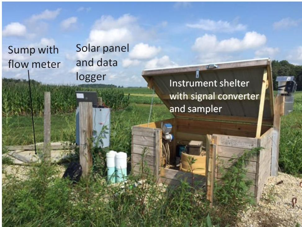
Figure 4: Research infrastructure for collecting drain flow, precipitation, wind speed, and water samples. Data are transmitted via a cellular modem. Soil moisture and water table measurements are also collected, but are within the field itself and are not shown here.
