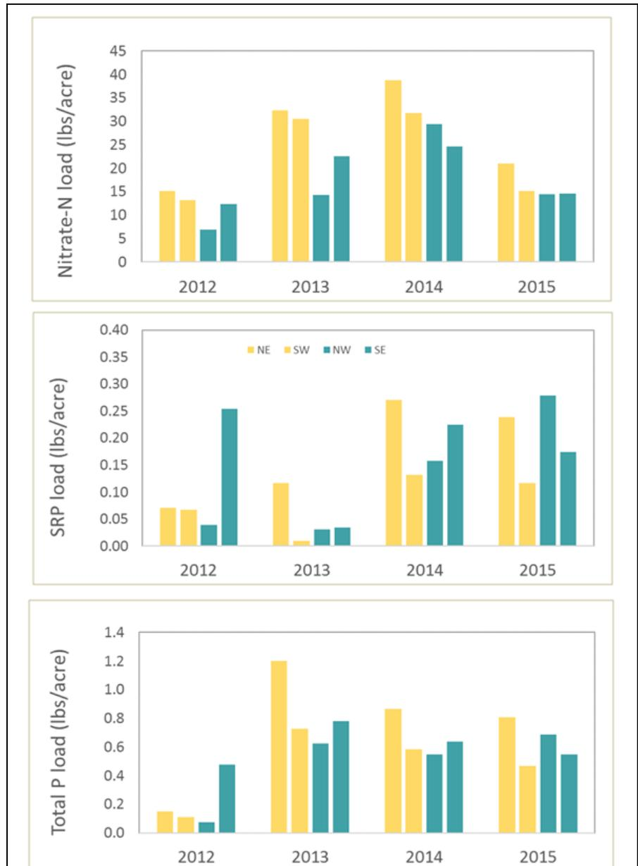
Figure 6: Loads of nitrate-N, soluble reactive phosphorus, and total phosphorus from free (gold) and drainage water management (aqua).
