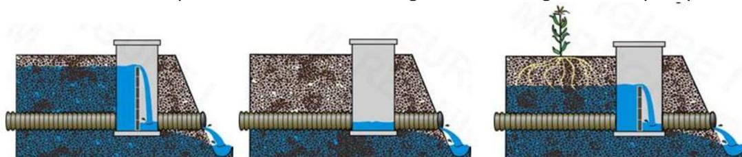
Figure 1: In drainage water management, the tile drainage outlet is raised after harvest to reduce nitrate delivery (left), lowered before planting and harvest to allow the field to drain fully (center) and raised again after planting to potentially store water for crops (right).
