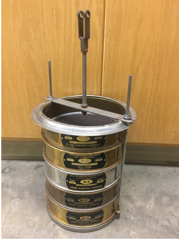
Stacked sieves used to collect different fractions of soil for measuring aggregate stability.
