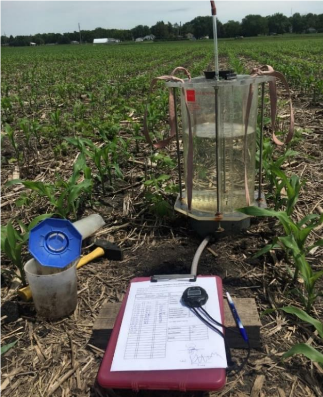
Cornell infiltrometer used to measure water infiltration in the field.
