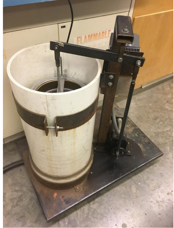
Motor and reservoir with stacked sieves inside for measuring aggregate stability.
