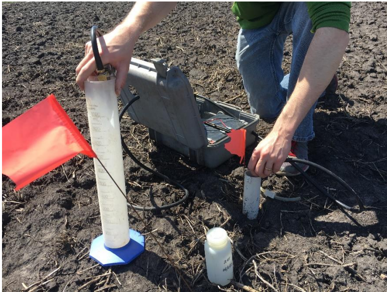
Using a vacuum pump to collect water from a lysimeter.
