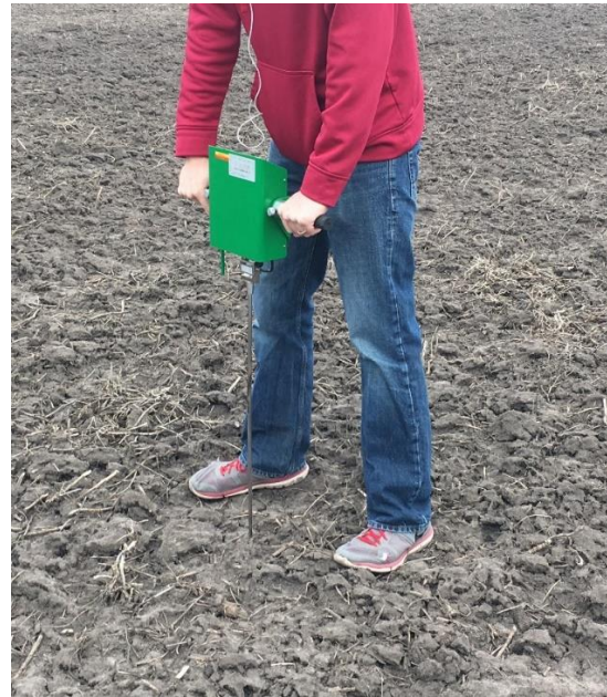
Rimik CP-20 Penetrometer for measuring soil compaction in the field.
