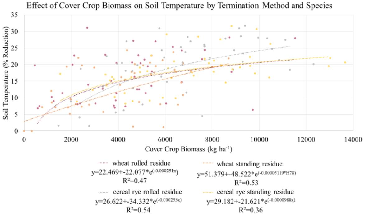
Figure 6. Effect of cover crop biomass on reduction in average soil temperature reduction relative to the no-cover check from cover crop termination to 6 weeks after by termination method (rolled versus standing) and cover crop species (cereal rye or wheat).
