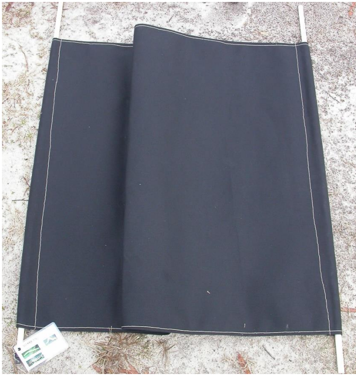
Fig. 7. Beat cloth and accompanying insect threshold card produced by the Taylor laboratory.
