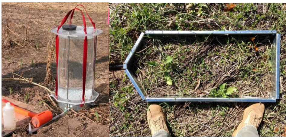
Figure 4 (Left) A Cornell Rainfall Simulator set up to measure infiltration and runoff and collect runoff samples. (Right). A mini-erosion weir installed in a 3-species cover crop that was interseeded into no-till soybean before harvest. The weir collects runoff from natural rain events on a 0.31 m 2 area. The tube on the left carries the runoff and sediment to a 2-gallon buried jug located 1 m downslope from the weir. An initial set of nine of these weirs were installed in October 2018 in anticipation of this project.
