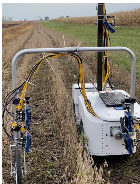
Figure 2. Field imaging of soybean pods using PhenoStereos and PhenoBot.
