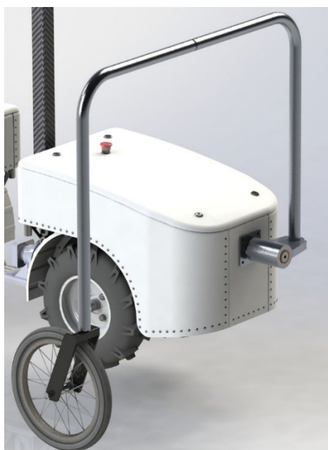
Figure 1. CAD model of the gate-shaped camera rig mounted at the rear of the Phenobot.
